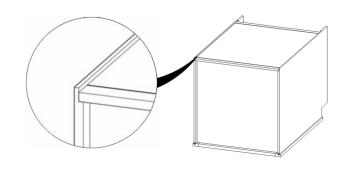
11. INSTALL DIVIDER ASSEMBLIES BY SCREWING THEM TO THE CABINET SIDES. (SCREWS NOT PROVIDED)
