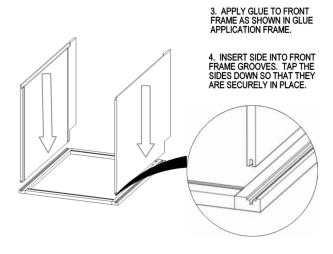
5. APPLY GLUE TO FEMALE DOVETAIL ON SIDES AS SHOWN IN GLUE APPLICATION FRAME.
